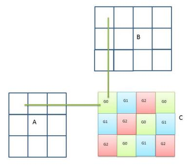
Figure 1 Example of cublasXt<t>gemm() tiling for 3 Gpus
