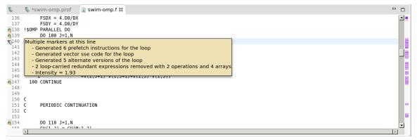
The CPU source code view allows you to inspect the files that comprise the profiled application's CPU source. This view can be opened in the CPU Details View by doubleclicking on a function in the tree–the source file that corresponds to this function is then opened. Line numbers can be enabled by right-clicking left side ruler.
